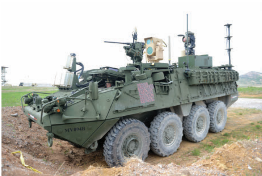
The U.S. Army is accelerating the prototype fielding of the Multi-Mission High Energy Laser, or MMHEL, which provides 50 kilowatt-class lasers on a platoon of Stryker combat vehicles by late 2022.
