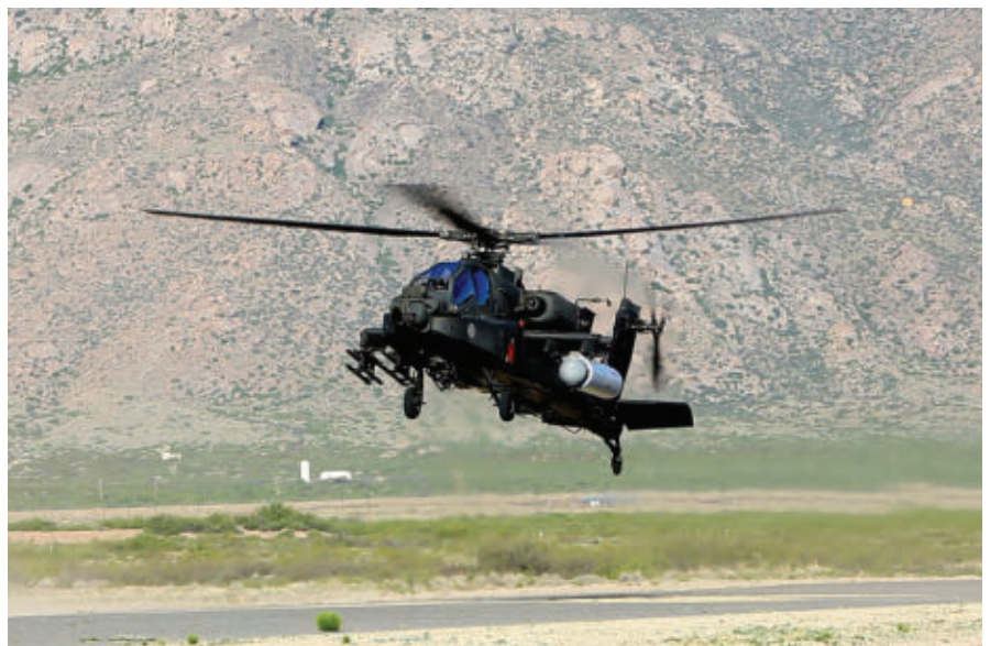
Raytheon, in partnership with the U.S. Army and U.S. Special Operations Command, has mounted a high-energy laser on an AH-64 Apache attack helicopter.
